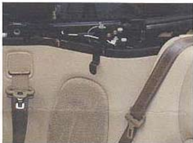
Fig:4 Interior view of larger piece of angle iron fitted correctly (driver's side)
