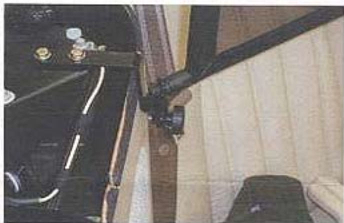
Fig:7 Fitting of large section of wind deflector through smaller piece of angle iron into larger piece of angle iron and held by thumb screw (driver side)
