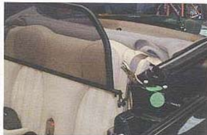
Fig:8 View showing test placement on passenger's side of wind deflector through pieces of angle iron prior to drilling. (held by clamp)
